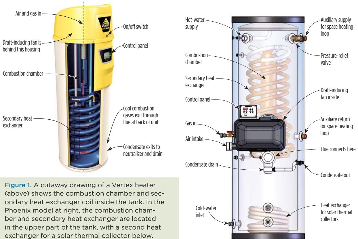
**Figure 1.** A cutaway drawing of a Vertex heater (above) shows the combustion chamber and secondary heat exchanger coil inside the tank. In the Phoenix model at right, the combustion chamber and secondary heat exchanger are located in the upper part of the tank, with a second heat exchanger for a solar thermal collector below.
