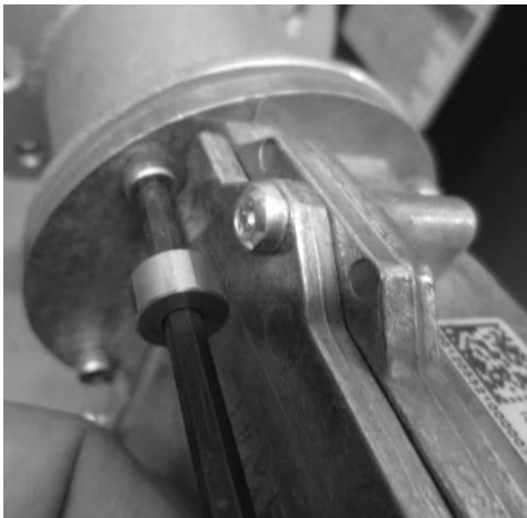
Figure 9 – Disconnecting Air Inlet Channel
