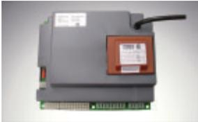
The **Munchkin 926 Control Board** is engineered to modulate the firing rate to match the actual needs of the heat system, saving money by conserving energy.
